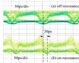
Fig. 4: Eye diagrams of star-16QAM when (a) off resonance and (b) on resonance, respectively.
