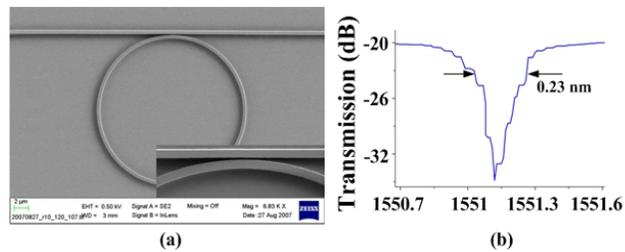
Fig. 2. The SEM photograph (a) and the measured spectrum in the through channel (b) of the microring resonator.
