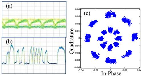
Fig. 3: Eye diagram (a), temporal waveforms (b), and constellation (c) of the star-16QAM
